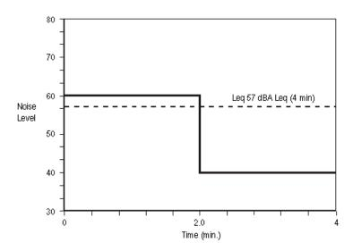
Figure 3 - Illustration of Leg concept
