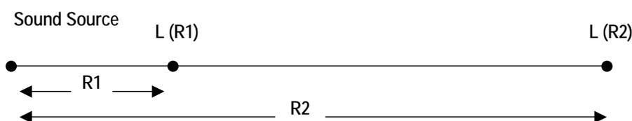
Note that the second term in the equation is negative if  $R_2$  is less than  $R_1$ , and  $L(R_2)$  is higher than  $L(R_1)$ . Also, under certain source-receiver configurations, the loss per doubling of distance can be less than six dB.
