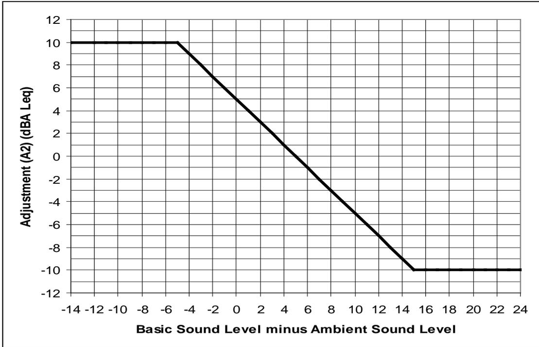
Figure 1 - Ambient monitoring adjustment, Class A2 adjustment
